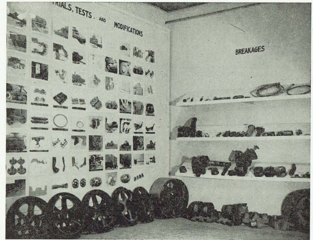
Defective bogie wheels and other mechanisms are turned in to the Experimental Wing for testing.
